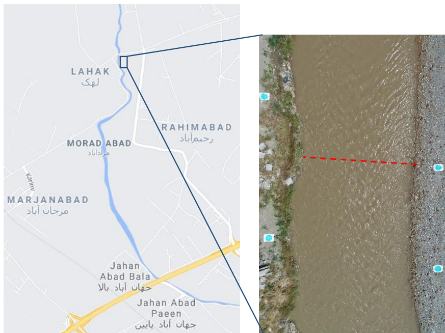
Fig 1. Location and an aerial image of the study area. The blue circles and the red dashed line on the right hand image show location of the GCPs and the surveyed cross section.
